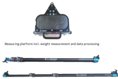
Ruler for track width measurement
